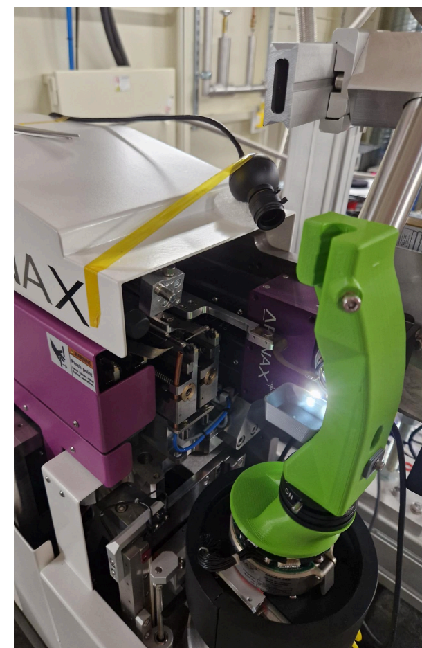
3D-printed HVE-injector holder on kinematic mount
